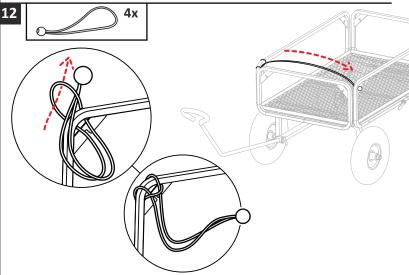
\* BALL END OF BUNGEE CORD CAN ATTACH TO ANY CORNER SLIT AS INDICATED ABOVE
