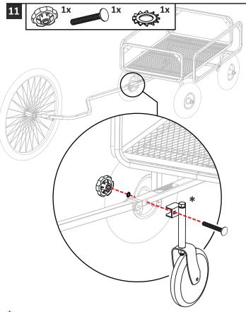
\* THE AIRPLANE NOSE WHEEL IS PROVIDED FOR ADDITIONAL STABILITY WHEN TURNING. SKIP STEP FOR BASIC KIT, IF USING THE BIKE ATTACHMENT OR ADDITIONAL STABILITY IS NOT NEEDED.
